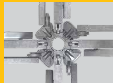
The node area offers 12 connection possibilities. In addition to four Ledgers and Node Braces respectively, four Ledger Braces can be connected.
